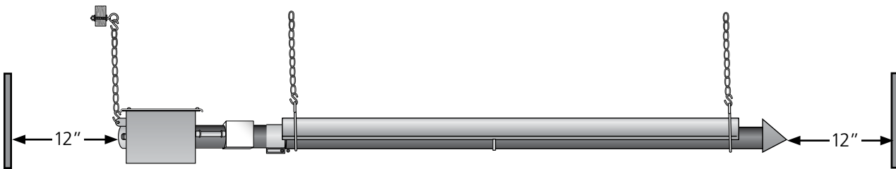
Figure 2.26 • Minimum end clearance for unvented heater
