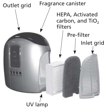
Figure 6 – Model 2HPD5A Air Purifier Parts
