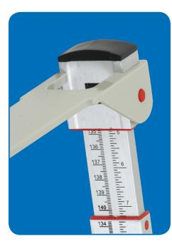
The red line on the height rod ensures easy and accurate height measurements.
