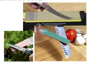
• Establish same angle as knife bevel with whetstone. 20° for most knives. Sharpen into the edge.
