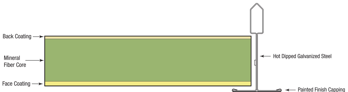
Figure 2. Composition of Prelude XL Suspension Systems
