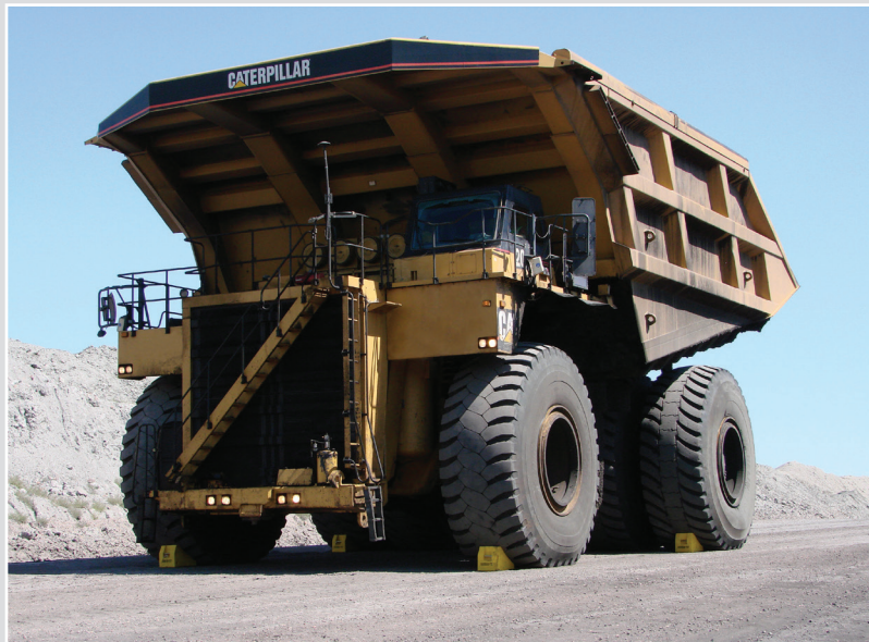
Four Monster wheel chocks, model 2IZF81 used on CAT 797
