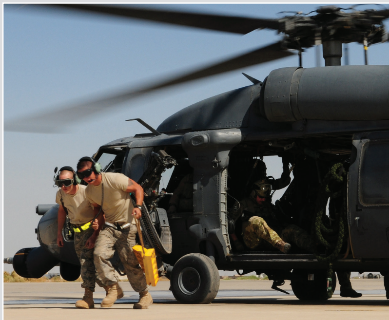
Monster aviation chocks model 5NHR9 used with HH-60G Pave Hawk
