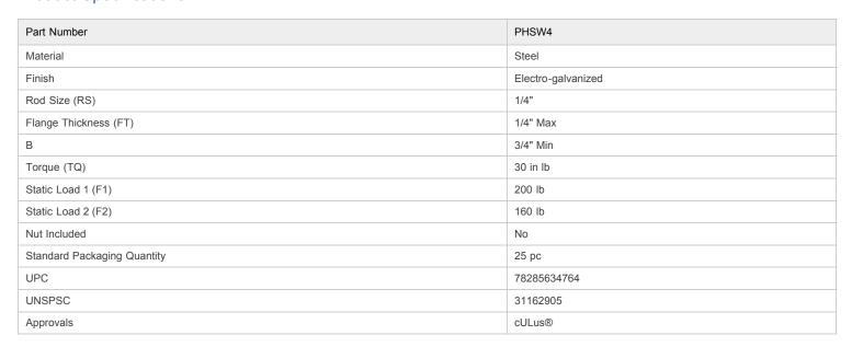
A jam nut is required for fire protection applications.
