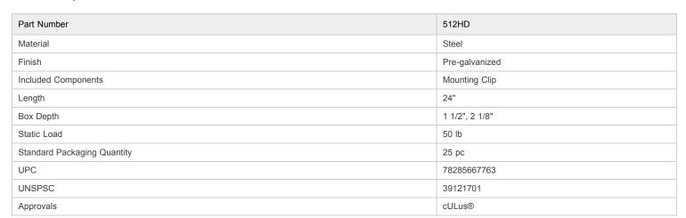
Standard bar mounts 2 1/8" box. Break off tabs for 1 1/2" deep box. Mounts flush with face of tile.
