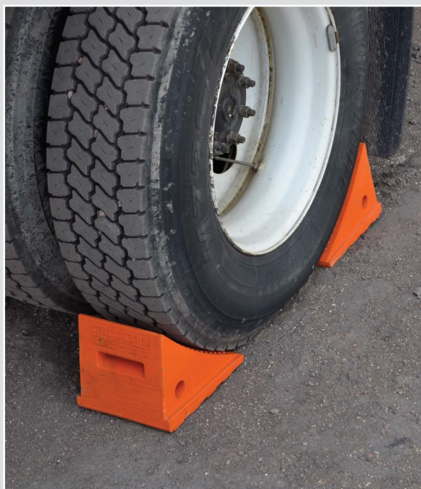
Monster urethane chocks model 28YL34 used on a utility truck
