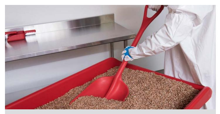
Remco shovels and scoops are made from durable and lightweight polypropylene and won't damage equipment, unlike metal tools. Remco tubs and undercarriages are ideally designed for many bulk material handling jobs that require containers made of FDA-compliant materials. Constructed with high-density polyethylene, they can be used for transporting, freezing, and storing.
