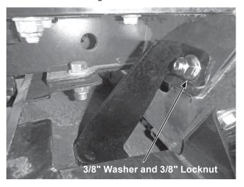
Repeat on the opposite side to install the passenger-side mount bracket. 6. Position the skid plate against the lower brush guard as shown, with the fastener holes aligned. Install four 3/8" x 1-1/2" cap screws through the skid plate, brush guard, and mount brackets. Install 3/8" washers and 3/8" locknuts to the cap screws and hand tighten.
