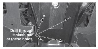
9. Install the four U-bolts over the frame and through the holes in the splash pan and skid plate.
