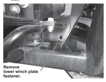
2. Remove the four lower brush guard support bracket fasteners.
