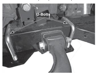
10. Secure each U-bolt with two 3/8" locknuts. Tighten according to the torque chart.
