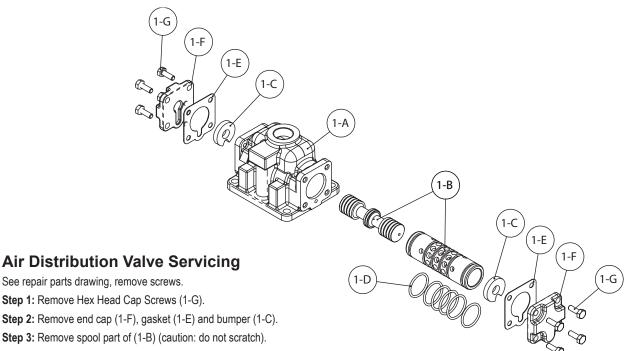
See repair parts drawing, remove screws.
