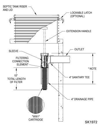
Zoeller Pump Company septic tank effluent filters are designed to protect all downstream components from solids. Every filter comes standard with bypass protection which keeps the filter working, even during cleaning!
