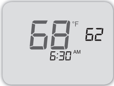
Figure 25. Thermostat Display shows temperature from Zone Sensor if working properly.
