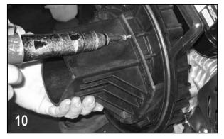
Install volute (12702A/13702) onto rear bracket using the three volute screws (12900/12725). Install check valve (12705) onto the snout of the volute. Drive unit should be turned over a few times to check for clearance between the two. A small amount of drag between impeller and volute is ok, however, if the drive unit will not turn over because of the lack of clearance, a bracket shim may have to be used.
