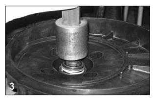
To install the carbon seal (12713) half into the rear bracket use a tool such as a 1  $\frac{1}{2}$ " pipe nipple or arbor press to give even pressure on the metal flange of the seal housing during installation. Gently press the seal into position until it bottoms.
