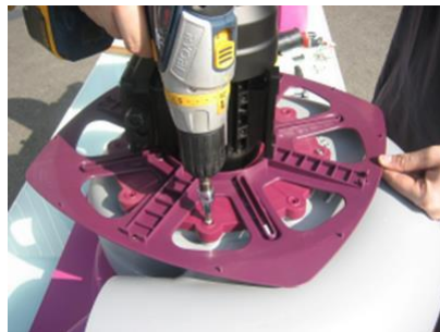
14-17. Screw the motor flange and the cap bracket on the housing indicated in the pictures.
