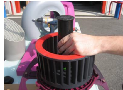
6. Push in the impeller.
