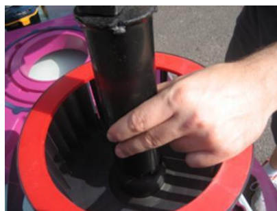
8. Install the hub cap.
