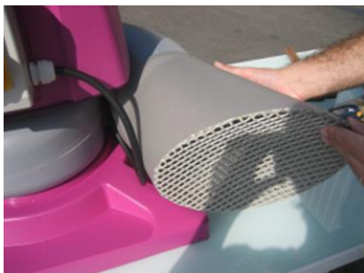
25. Place the exhaust cap on the outlet and attach with 4 screws.
