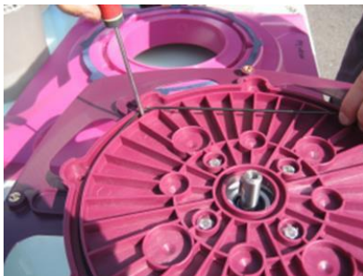
4. Place the O-ring seal.
