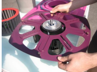
2. Place the cap bracket on the motor with the screwing inserts upwards.
