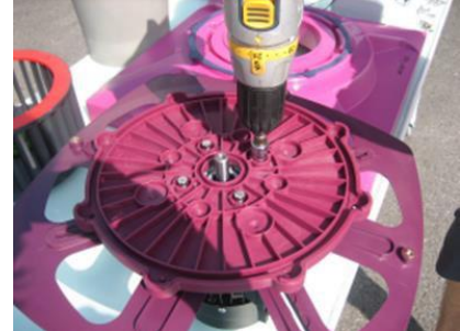
3. Fix the motor flange.
