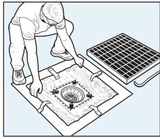
4. Place Filtration Insert System directly on grate lip inside of storm drain.
