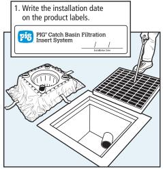
2. Remove drain grate and clean any existing sediment off grate lip inside of storm drain.
