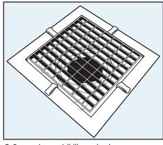
7. For maximum visibility and to keep system securely in place, ensure green straps are not caught beneath storm drain grate.
