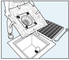
3. Expand or collapse frame to fit intended storm drain size.
