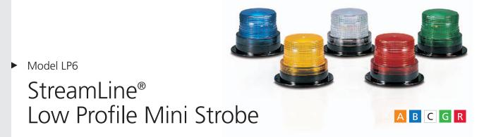
The Model LP6 is a very compact, high power strobe light designed for applications where space is critical. At 3-5/8" high, this strobe light is ideal for forklift applications where head room is important. The LP6 also mounts easily to small control panels.
