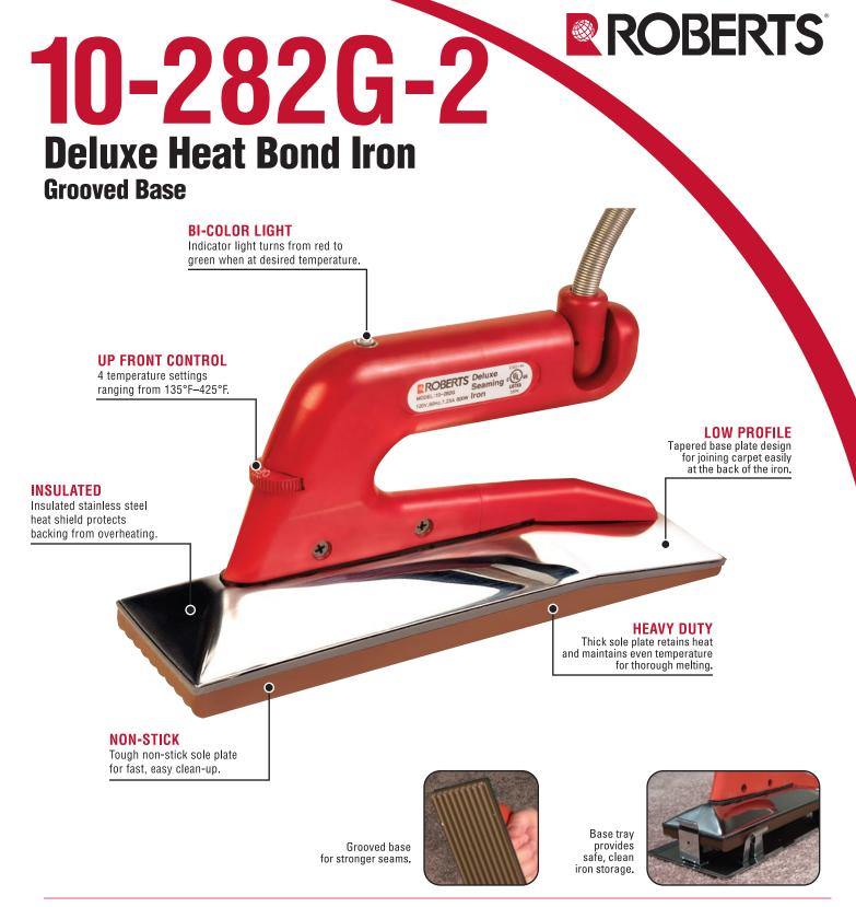
The Roberts Deluxe Carpet Seaming Iron has an adjustable thermostat and heat shield to provide ideal heat for hot melt tape while protecting carpets from high temperatures. Streamlined, low profile design provides even heat distribution for thorough melting and easy carpet seaming. This iron has a heat range of 135°F to 425°F.
