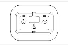
If new mounting holes are needed, mark the placement of the new horizontal mounting holes through the trim plate base. Using a 3/16" drill bit, drill the holes you have marked and insert the supplied wall anchors.
