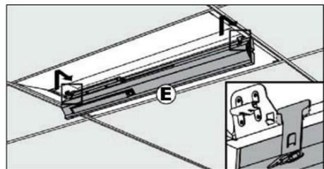
**12** Maneuver the Light Engine (E) in the slots of one of the two Closing Panels (C). The design of the Closing Panel (C) prevents the Light Engine (E) of falling out during electrical and ground connection (see detail).
