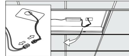
**4** Disconnect host fixture ballast from mains.
