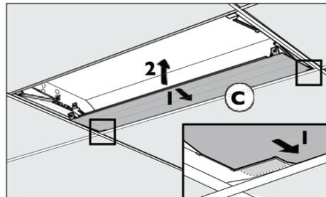
**8** Install Closing Panel (C) in between troffer and T-grid, making sure the tabs at each corner of the LED panel slide into the respective slots on the side panel.
