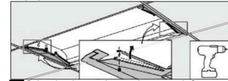
**7b** EvoKit end panels come with integrated securement tabs. Securement tabs can be affixed to existing troffer housing with self tapping screws (not provided). Additional earthquake tabs can be purchased if required (502435).
