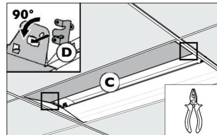
**11** Push Closing Panel (C) upward into position until tab engages into slot to temporarily secure. Fixate panels and establish ground by turning each fastener (D) 90 degrees.
