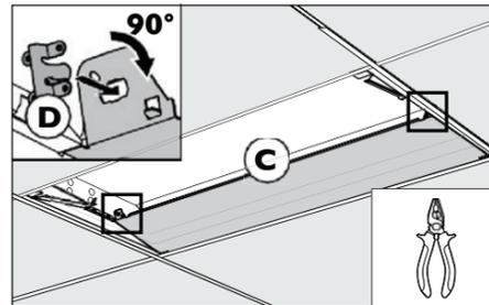
**9** Push Closing Panel (C) upward into position. Secure panels and establish ground by turning each fastener (D) 90 degrees.
