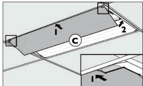
**10** Install Closing Panel (C) in between troffer and T-grid, making sure the tabs at each corner of the Closing Panel slide into the respective slots on the side panel.
