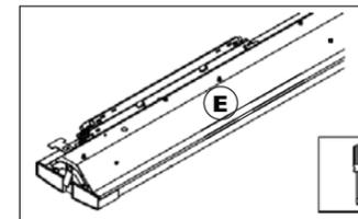
Optional mounting holes for installing a compatible Philips/Bodine Emergency LED Driver are located on the Light Engine (E). The distance between the mounting holes is ~414 mm.
