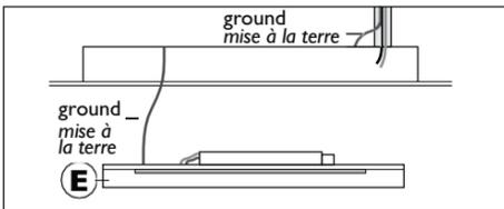
**13a** Situation 1 Grounding: Screw grounding cable from Light engine (E) to original troffer if host fixture ground connection is made through host fixture.
