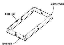
1. Cut ceiling opening to proper dimensions. Slip fit corner clips into side and end rails. No tools are required.
