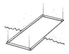
2. Place Flange Kit in ceiling opening and wire each corner to ceiling structure. Pull up tight against ceiling.
