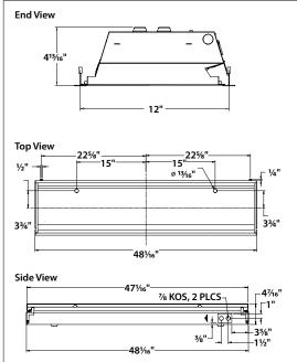
A: %" Diameter knockout K: 2" × 3" through hole for access plate.
