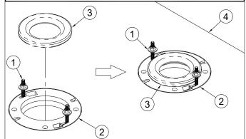
Remove Fixture Access Panels. Align fixture outlet over Closet Flange and against wall, setting fixture on the floor firmly in place onto Closet Flange and T-Bolts. Secure Closet Flange.
