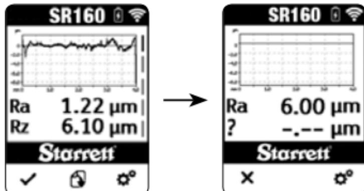
In the calibration screen, the default or last saved calibration Ra value will be displayed. To change this calibration value, press the settings icon. Then use the up (+) and down (-) buttons to adjust the calibration Ra value to the desired number. Press the back button to accept the value and return to the calibration screen.
