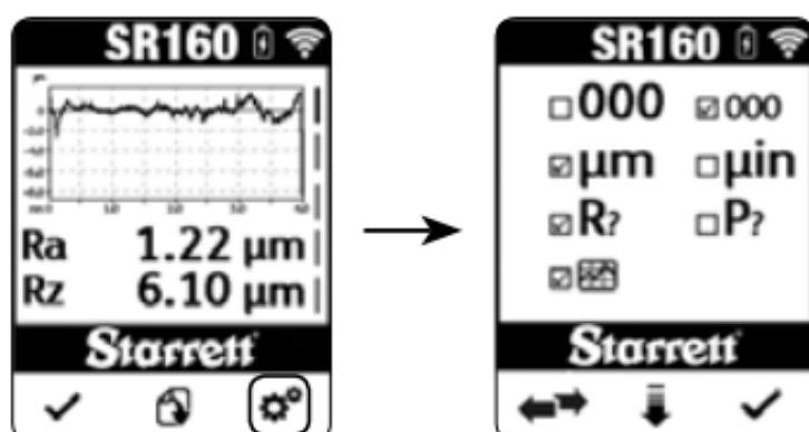
Press the down arrow button to scroll down to the Graph option line. Press the to toggle between the option of displaying or not displaying the graph on the results screen. Press the check button to accept the setting and exit the settings menu.
