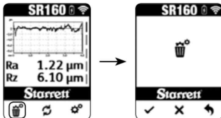
The factory reset function works only when the SR160 is paired (either via Bluetooth or in connected mode).
