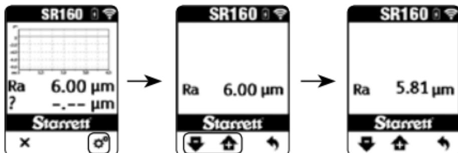
Place the SR160 on the calibration standard provided with the unit (or any other certified standard). Press the measure button to take a measurement on the calibration standard.
