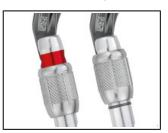
To facilitate equipment checks, SCREW-LOCK manual locking carabiners have a red band that is visible only when the carabiner is not locked.
