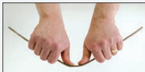
Brake tubing can be easily bent by hand
