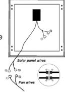
wire from the solar panel to the positive wire from the fan, and the negative wire from the solar panel to the negative wire from the fan.
