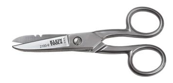
These Klein Tools Cable Splicer Snips cut 19 AWG and 23 AWG electrical wire, cable and cordage. The stainless steel blades maintain sharpness and durability. Serrated teeth provide non-slip cutting action. The snip has a free-fall feature for ease of use.
