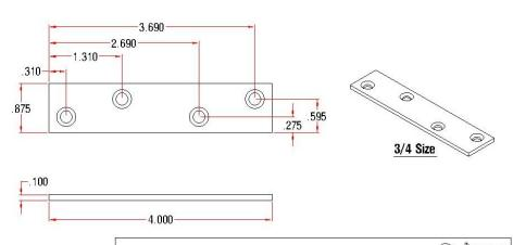
Material: 1018 Steel Finish: Zinc Plated Plates must be preped to dimesions shown for a #8 Philips Flat Head SMS.
