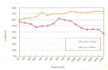
LnO,W (uncoated slab)= 79 dB (according to EN ISO 717-2: 1996)
