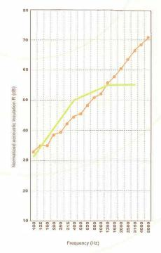
Insulation index to airborne sounds: R<sub>w</sub> (C; Ctr) = 51 (-2; -6) dB
