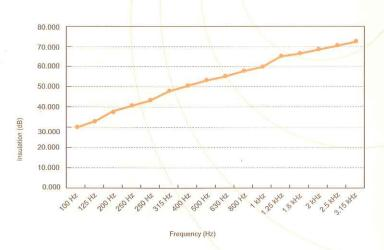
Insulation index to airborne sounds: Dn,w = 55dB
