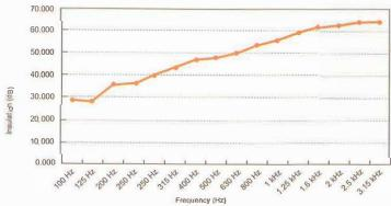
Insulation index to airborne sounds: Dn,w = 50dB
