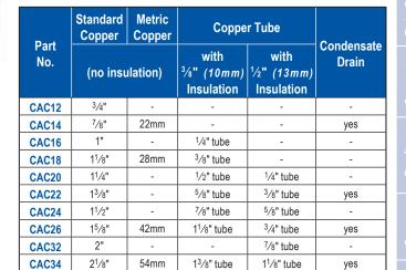
Inside diameter: Certain clips have two or more positions to accommodate both metric and standard sizes
