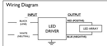
Input & Output use 18AWG 105C/600V solid copper lead wires
