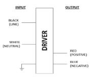
Input and output use lead- wires. Lead-wires are 18AWG 105C/600V solid copper. Input Lead Length outside enclosure: 9" (+2"/-1"). Input Lead Length outside enclosure: 26" (+2"/-1"). Driver case must be grounded.
