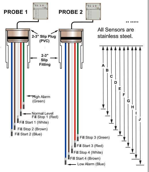
Dimensions should be calculated from the top of the tank or riser down to the required alarm level(s) in inches. Be sure to take into account any riser pipes or manway risers.
