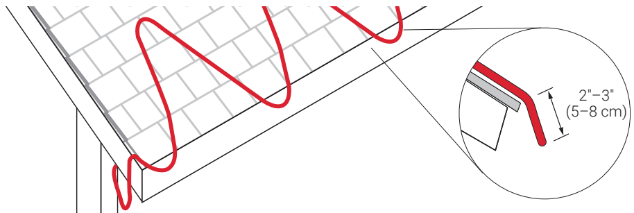
Figure 6 Layout for heated drip loops
