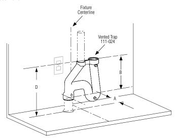
\* Suggested location of 120VAC GFCI electrical outlet. Always check local codes before installing. Outlet may be required to be in a remote location.
