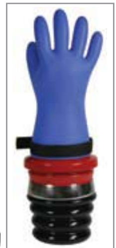
G100 with inflated lo-volt glove ready for inspection.
