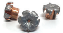
.40 Caliber Rounds stopped in SAC-D from 10 Yards
