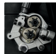
Heavy-duty aluminum two-drive-roll system
