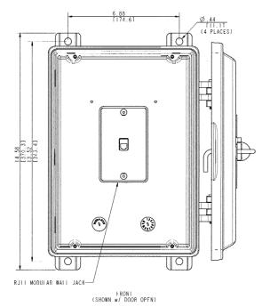
**Note: Dimensions in Brackets** are in Millimeters.
