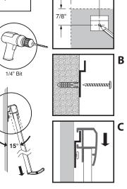
Insert screws through hanging brackets into the wall anchor (B). Tighten firmly. Holding the board at
