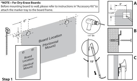
Determine board location. To position top hanging brackets, mark center hole of hanger 6" from outside edge of board and 1-3/8" down from top of board (A). Drill holes for each hanger in marked locations using a 1/4" drill bit. Insert wall anchors into holes flush with the wall.
