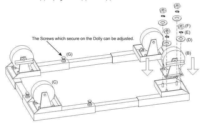
Step 2. To loose all the screws and adjust the length & width which you want.
