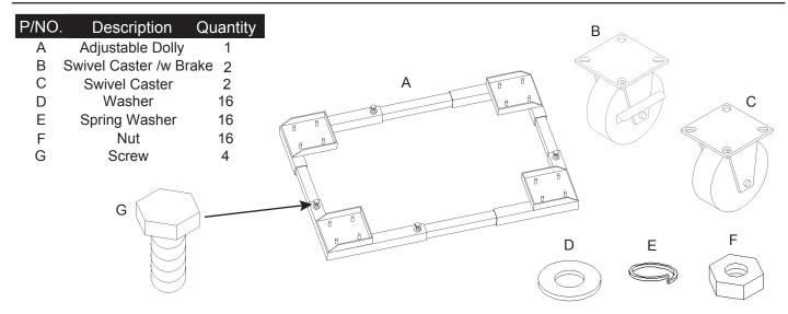
Step 1. Place the Swivel Caster /w Brake (B) & Swivel Caster (C) on the back of Adjustable Dolly (A), and secure it with Washers (D) & Spring Washers (E) and Nuts (F).
