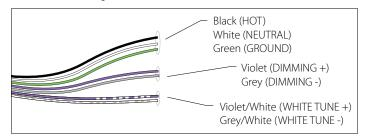
SpectraSync Tunable White luminaires are provided with two 0-10V circuits. The violet and grey circuit is for wiring to any qualified 0-10V controller for dimming. The violet/white and grey/white circuit is for wiring to any qualified 0-10V controller for Tunable White CCT control.
