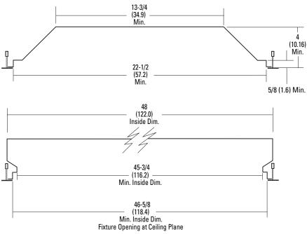
Relight assemblies are designed to fit most recessed fixtures mounted in T-grid installations. For surface mounted fixtures or for fixtures mounted in ceiling types other than T-grids, consult factory before ordering.
