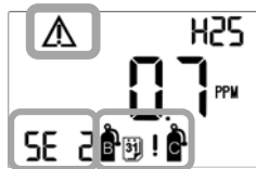
Single-sensor bump test failure
