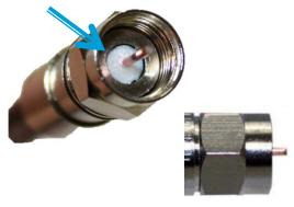
4) Cable is fully seated when white dielectric is flush with the bottom of the nut. Pin should slightly extend beyond edge of nut.
