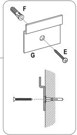
2 Elevate board at 30° angle and hook back frame channel into secured mounted **Z-Brackets**. Check that board is secure in place before releasing.
