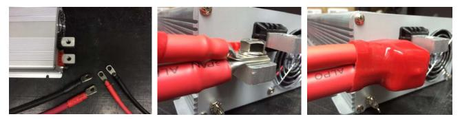
b. Install the "bare wire extremities" on the battery charger DC output receptacles. Each bare wire extremities must be inserted in the correct output receptacle.
