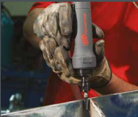
Weld cleaning and smoothing
